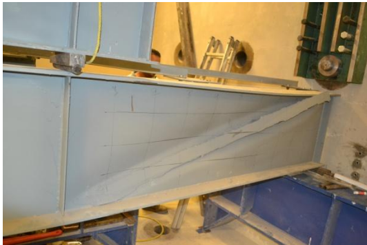
Figure 14: Web buckling and de-bonding of CFRP (SG-3.5-135-2)
