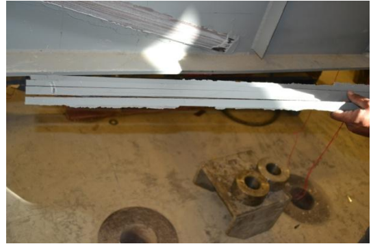
Figure 13: De-lamination in detached CFRP (SG-3.5-135-1)
