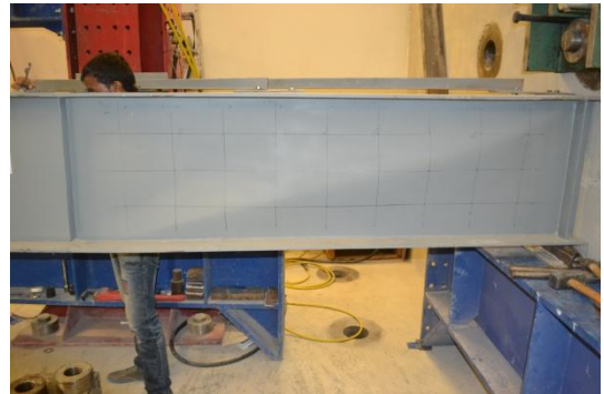
Figure 11: Web buckling and formation of tension fold (CG-3.5-135)
