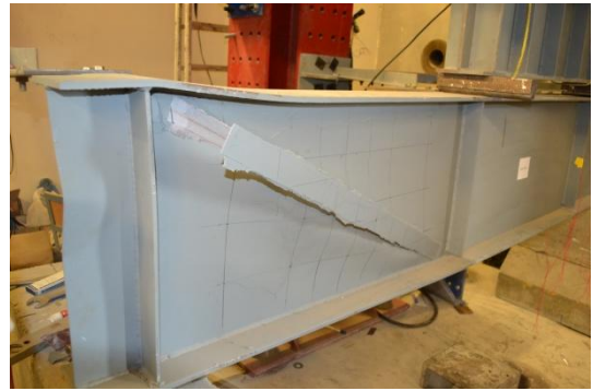
Figure 9: Web buckling and de-bonding of CFRP (SG-2-135-1)
